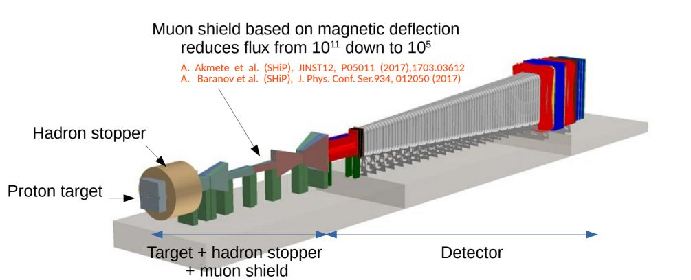
**Upstream detector** Scattering and Neutrino Detector (SND) designed for recoil **signatures of light dark matter scattering** and **for tau neutrino** physics.
