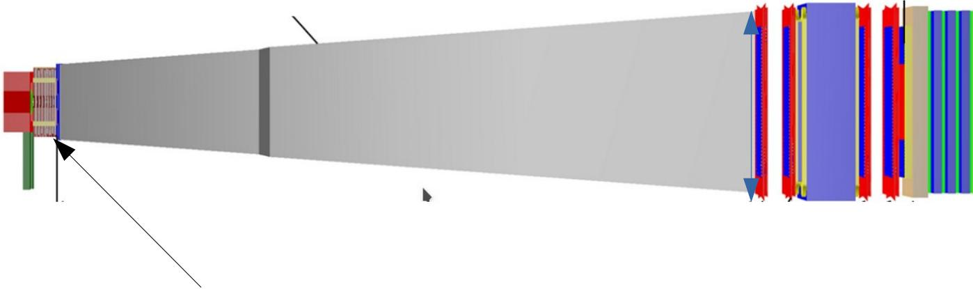
**Upstream Veto Tagger** with the purpose to veto events induced by neutrinos or muons in the vicinity of the entrance of the decay vessel is based in the **MRPC technology**.
