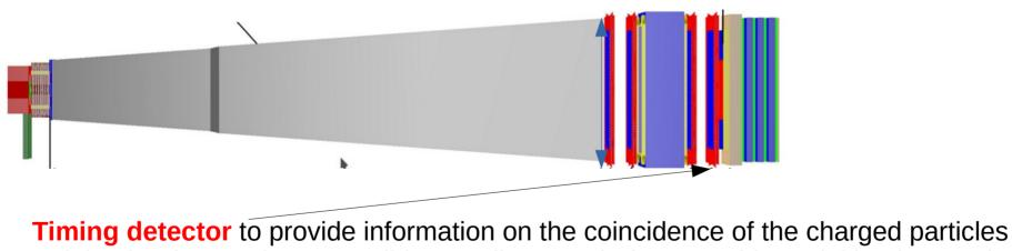
riginating from a decay candidate to disentangle from combinatorial background. Two technologies are proposed, plastic scintillators providing 80 ps σ. C. Betancourt, (SHiP), Nucl. Instrum. Meth. A979, 164398 (2020) and MRPC => LIP contribution, see later
