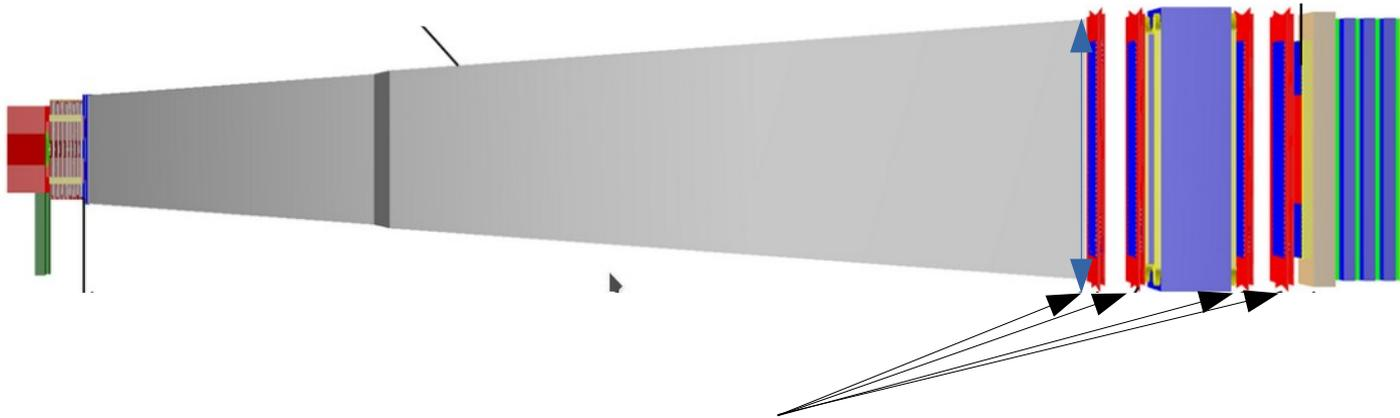
**Spectrometer Tracker**, designed to accurately reconstruct the decay vertex, the mass, and the impact parameter of the hidden particle trajectory at the proton target, includes four tracker stations, two stations upstream and two downstream of the magnet. The baseline technology are **straw drift tubes** 2 mm long, providing 120  $\mu\text{m}$   $\sigma$ .
