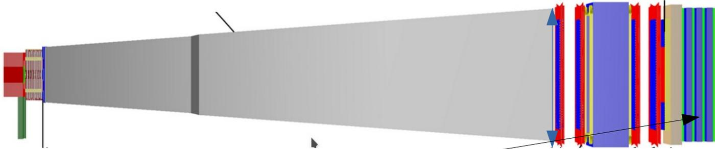
**Muon system** for the identification of muons comprise four stations of active layers, based on **scintillating tiles with direct SiPM readout**, interleaved by the three muon filters providing an efficiency detection >95 %.
