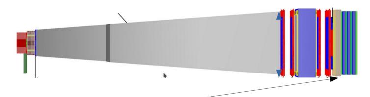
**Electromagnetic calorimeter** providing electron and photon identification and discrimination against hadrons and muons, as well as measuring the shower angle. It is based on a **segmented lead sampling calorimeter equipped with scintillating plastic bars** read-out by WLS fibers with course spatial resolution and high resolution planes based on **micro-megas**.
