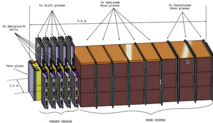
The muon detector has been replaced by scintillating technology and a veto plane added.
