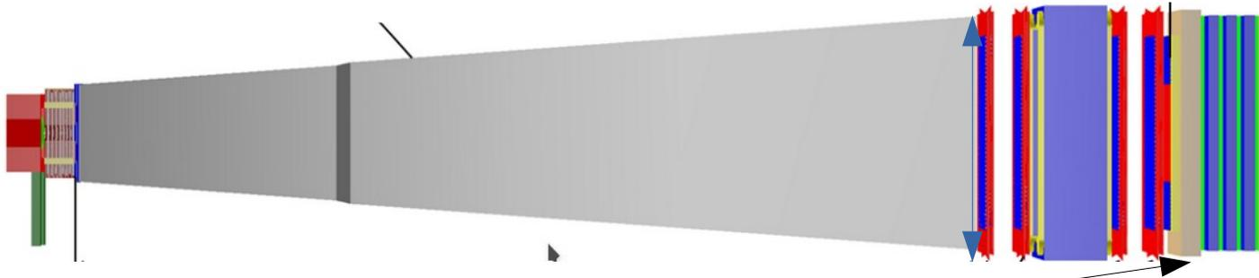
**Electromagnetic calorimeter** providing electron and photon identification and discrimination against hadrons and muons, as well as measuring the shower angle. It is based on a **segmented lead sampling calorimeter equipped with scintillating plastic bars** read-out by WLS fibers with course spatial resolution and high resolution planes based on **micro-megas**.
