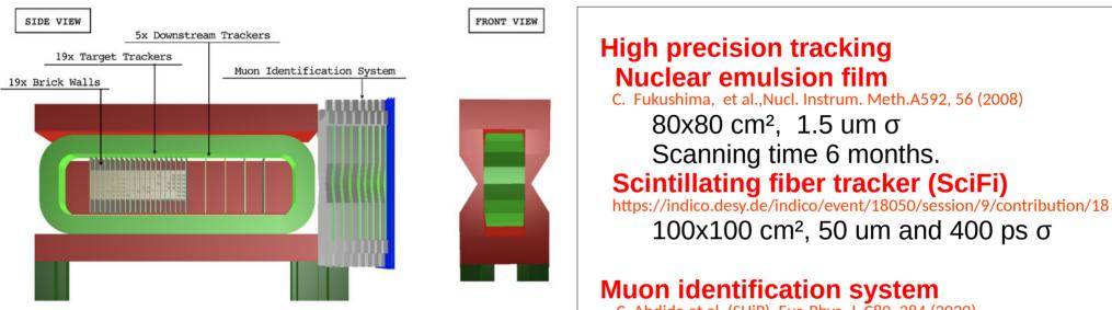
It consists of a spectrometer magnet housing a layered detector system with high-density target plates, emulsion film technology and electronic high precision tracking to determine the charge and momentum plus a muon identification system. Auon identification system C. Ahdida et al. (SHiP), Eur. Phys. J. C80, 284 (2020) Resistive Plate Chambers (Bakelite) 4300x2900 cm<sup>2</sup>, 1 cm strips
