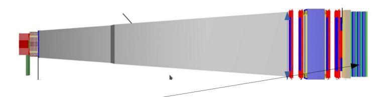
Muon system for the identification of muons comprise four stations of active layers, based on scintillating tiles with direct SiPM readout, interleaved by the three muon filters providing an efficiency detection >95 %.
