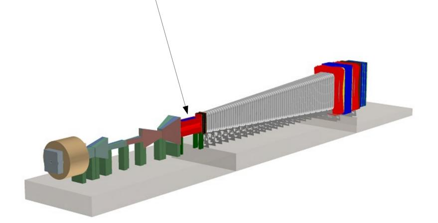
**Upstream detector** Scattering and Neutrino Detector (SND) designed for recoil **signatures of light dark matter scattering** and **for tau neutrino** physics.
