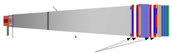
Spectrometer Tracker, designed to accurately reconstruct the decay vertex, the mass, and the impact parameter of the hidden particle trajectory at the proton target, includes four tracker stations, two stations upstream and two downstream of the magnet. The baseline technology are straw drift tubes 2 mm long, providing 120 um  $\sigma$ .
