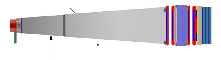
To ensure signal candidates, the decay volume is completely covered by a high efficiency background tagger system based on liquid scintillator technology readout by wavelength--shifting and SiPM, providing 99.9 % detection efficiency.
