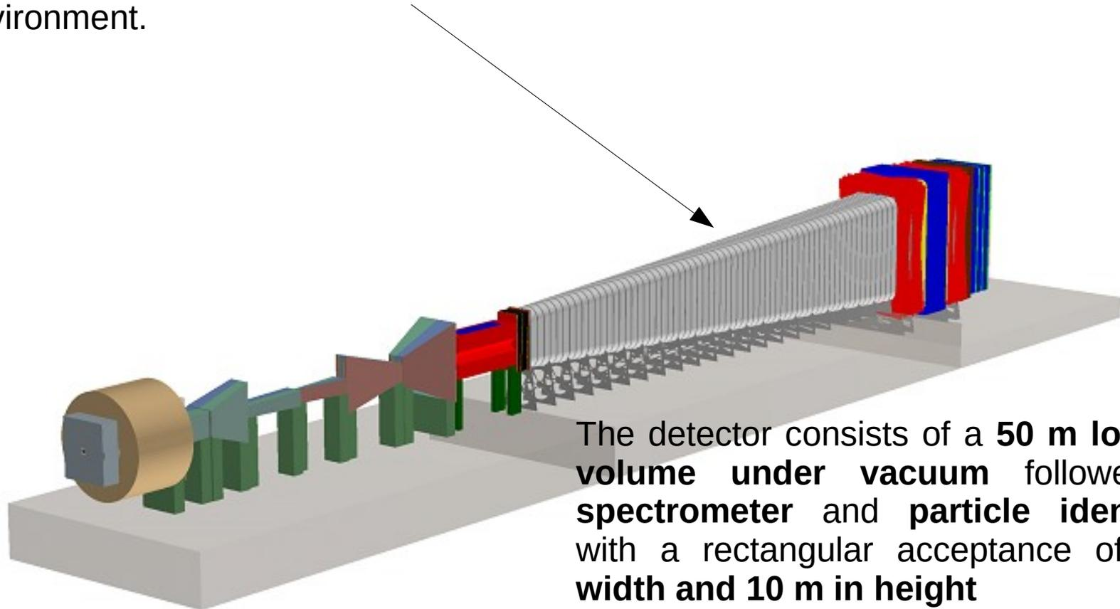
The detector consists of a **50 m long decay volume under vacuum** followed by a **spectrometer and particle identification** with a rectangular acceptance of **5 m in width and 10 m in height**
