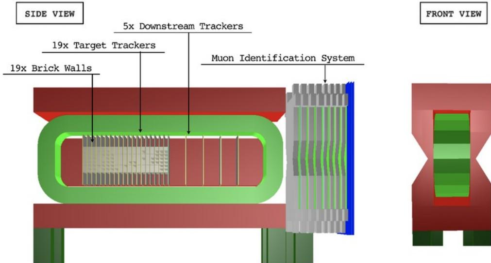
It consists of a spectrometer magnet housing a **layered detector system with high-density target plates, emulsion film technology and electronic high precision tracking to determine the charge and momentum plus a muon identification system.**
