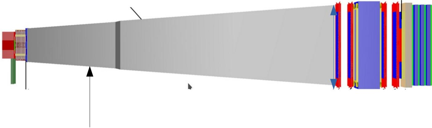
To ensure signal candidates, the decay volume is completely covered by a high efficiency **background tagger system based on liquid scintillator technology readout by wavelength--shifting and SiPM**, providing 99.9 % detection efficiency.
