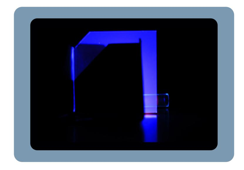
Figure 2 - Scintillating material
