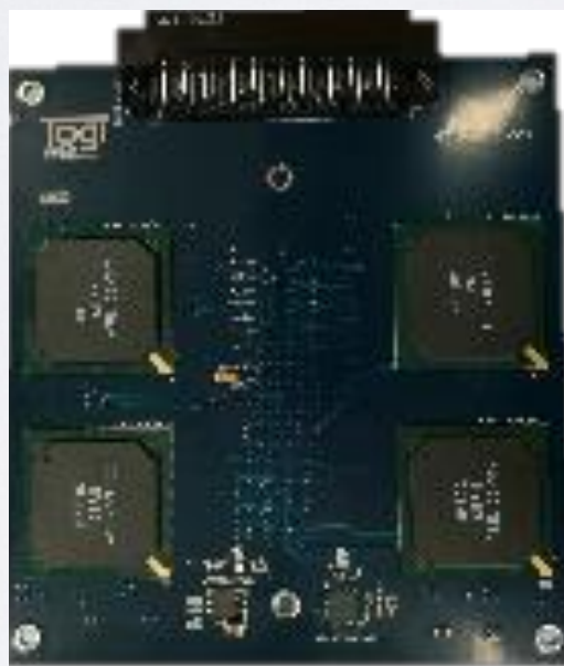
New time->digital converter cards for PPS (LIP-CMS design)
