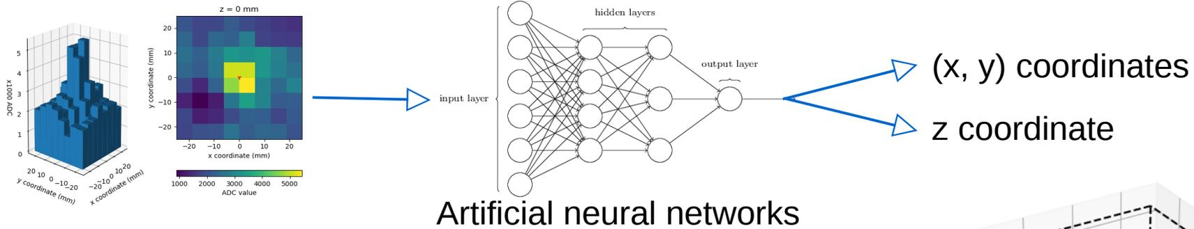
Position resolution is about **2.5 mm** at high enough energy ( $> 150$  keV) with an optimized neural network architecture (hidden layers design)
