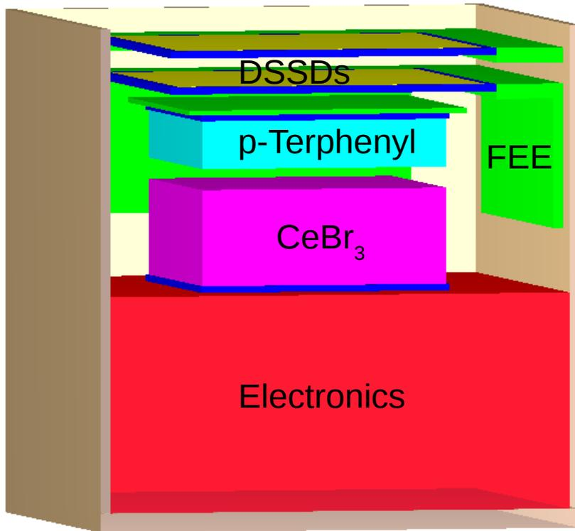
Adding a plastic (p-Terphenyl) based Anger camera increase the effective area at lesser cost than adding DSSDs
