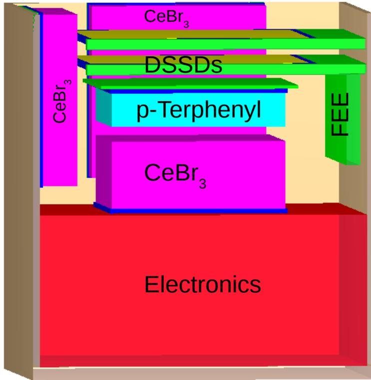
Adding thinner  $\text{CeBr}_3$  detectors on the sides help catching scattered gamma rays
