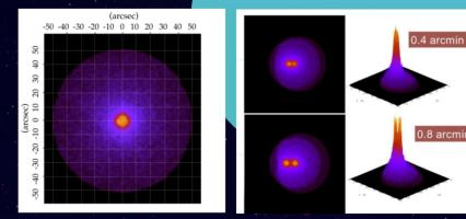
The Laue lens PSF simulated using the new SW tools for the case of a on-axis point source and two source a different angular distance in the Lens FOV.
