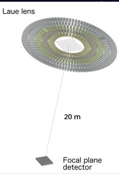
The Laue lens is made by bent crystals tiles distributed in concentric circles extending from 0.26 up to 3 m in diameter
