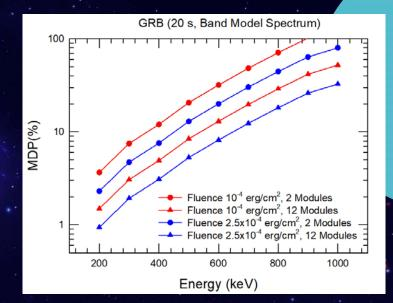
Minimum Detectable Polarization at 3 level for a GRB of 20 s duration and 2 different fluences. \* AD 2020 AHEAD Coimbra
