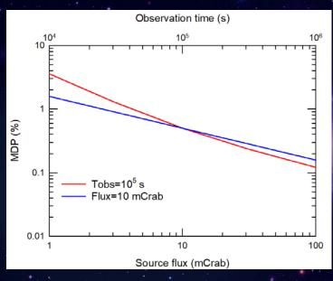
Minimum Detectable Polarization (MDP) in the full (50-600 keV) Laue lens passband, in 10<sup>5</sup> s, as a function of the polarized source intensity (red line) and, for a 10 mCrab source, as a function of the observation time (blue line).
