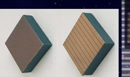
(right) The 3D CZT sensor: 20x20x5 mm<sup>3</sup>; Anode side: 12 collecting anodes,
