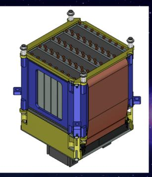
Overview of the the 8x8 CsI-SDD module with its ASIC AFEE under realisation as THESEUS XGIS demonstrator. The CsI bars are 3 cm long and 0.5x0.5 cm<sup>2</sup> section.
