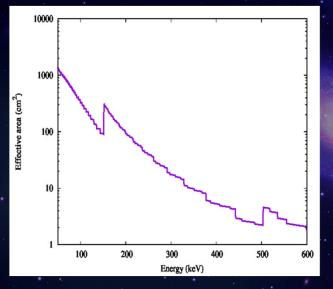
The ASTENA Laue Lens efficient area evaluation as a function of energy obtained with the improved sw tool
