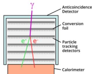
Fig. 7: Cross-section of the LAT. Credits: NASA's Goddard Space Flight Center.
