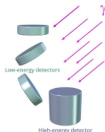
Fig. 8: Low-energy detectors on GBM face. Credits: NASA's Goddard Space Flight Center.
