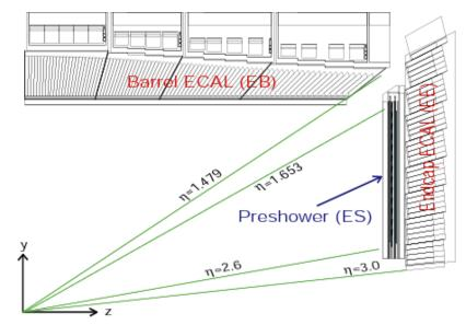
Electron and photon detection PbWO<sub>4</sub> scintillating crystals & avalanche photodiodes
