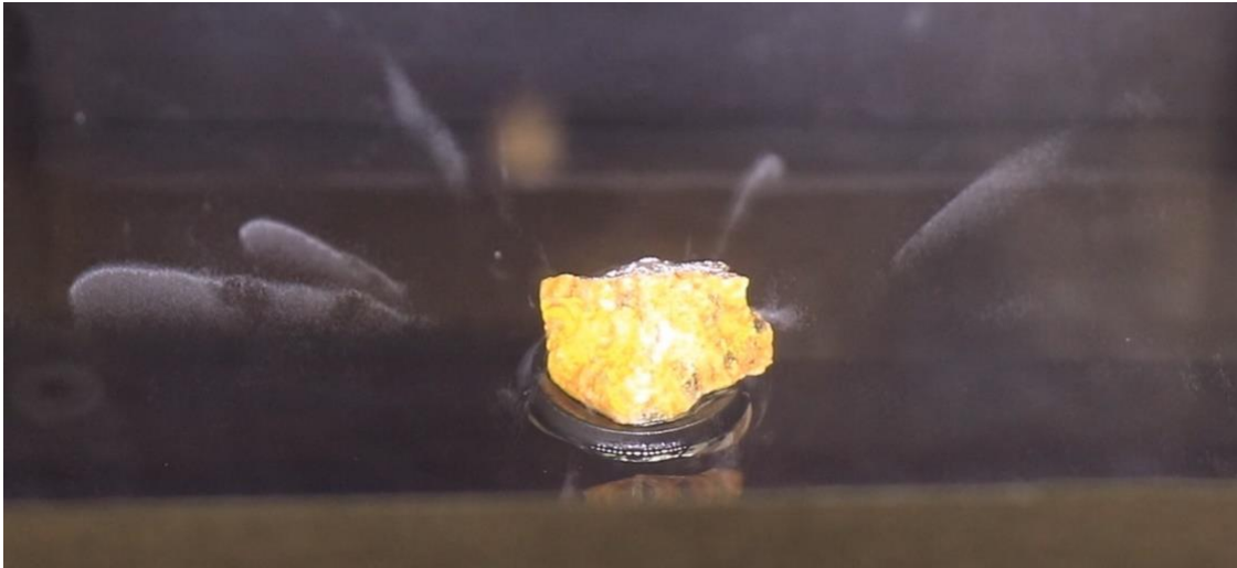
Tracks of alpha particles seen in a cloud chamber at LIP
