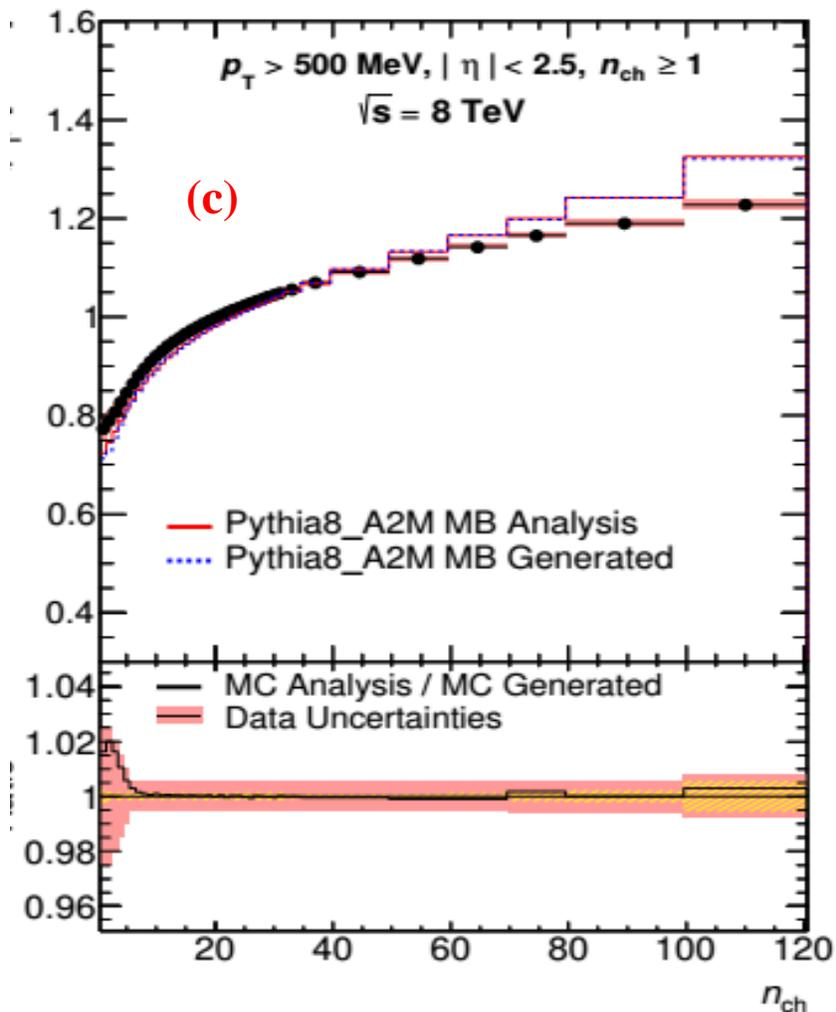
Average transverse momentum as a function of the number of charged particles in the event for events with  $n_{ch} \geq 1, p_T > 500$  MeV and  $|\eta| < 2.5$  at  $\sqrt{s} = 0.9$  (a), 7 (b) and 8 TeV (c). The dots represent the data and the curves the predictions from different MC models.
