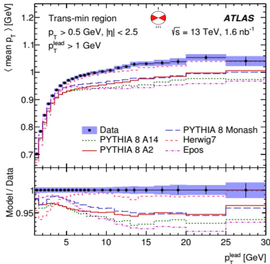
Mean charged-particle average transverse momentum as a function of charged-particle multiplicity in transverse region  $N_{ch}$  and as a function of  $p_T^{lead}$
