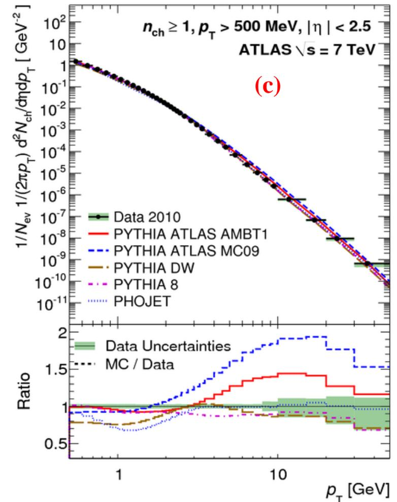
Charged-particle multiplicities as a function of the transverse momentum for events with  $n_{ch} \geq 1$ ,  $p_T > 500 \text{ MeV}$  and  $|\eta| < 2.5$  at  $\sqrt{s} = 0.9$  (a), 2.36 (b) and 7 TeV (c). The dots represent the data and the curves the predictions from different MC models.
