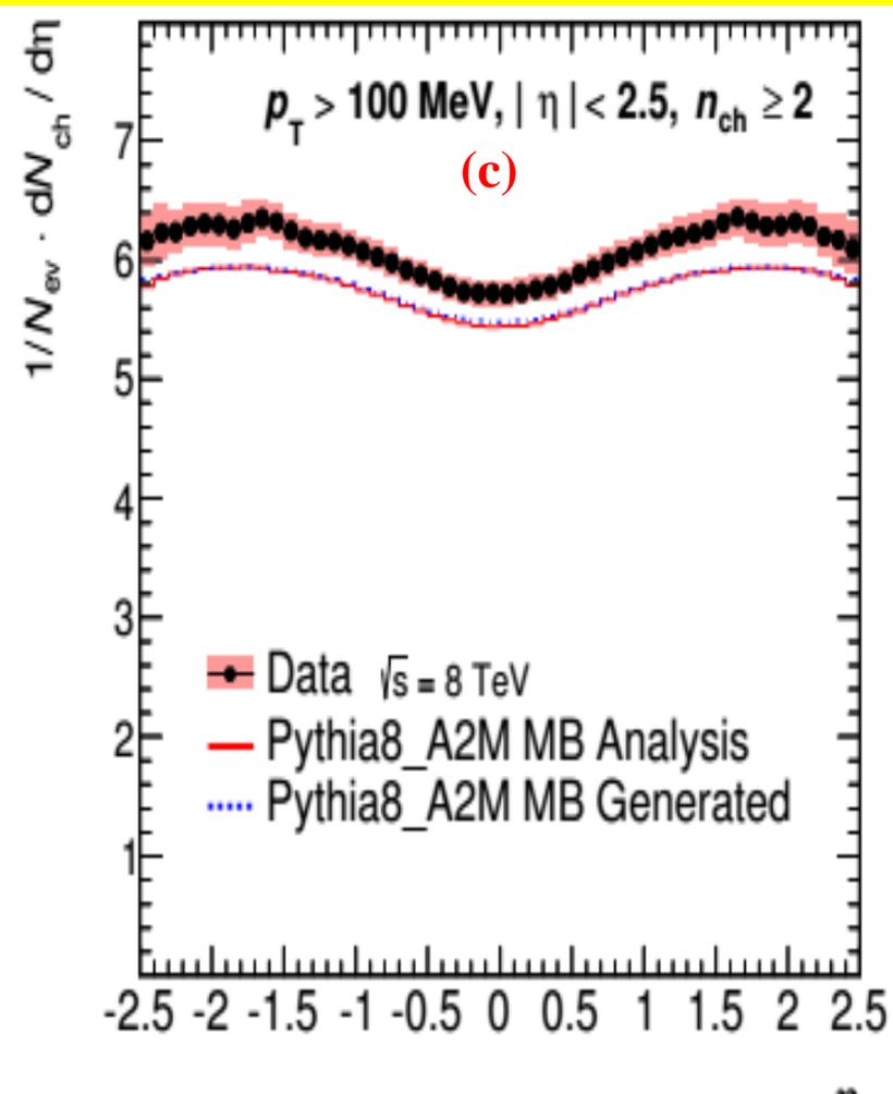
Charged-particle multiplicities as a function of the pseudorapidity for events with  $n_{ch} \geq 2, p_T > 100 \text{ MeV}$  and  $|\eta| < 2.5$  at  $\sqrt{s} = 0.9$  (a),  $7$  (b) and  $8 \text{ TeV}$  (c). The dots represent the data and the curves the predictions from different MC models
