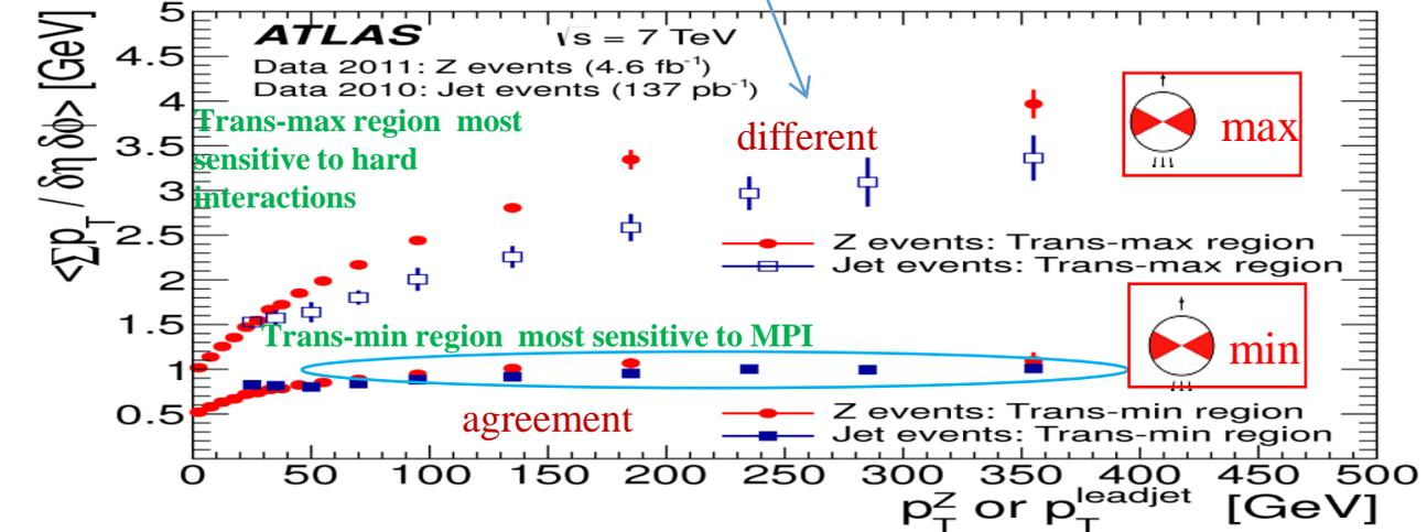
Charged particle multiplicity average values and scalar  $p_T$  sum density average values compared between leading charged particle ( $MB$ ), leading jet and Z boson events, respectively as functions of leading track  $p_T$ , leading jet  $p_T$  and Z boson  $p_T$ .
