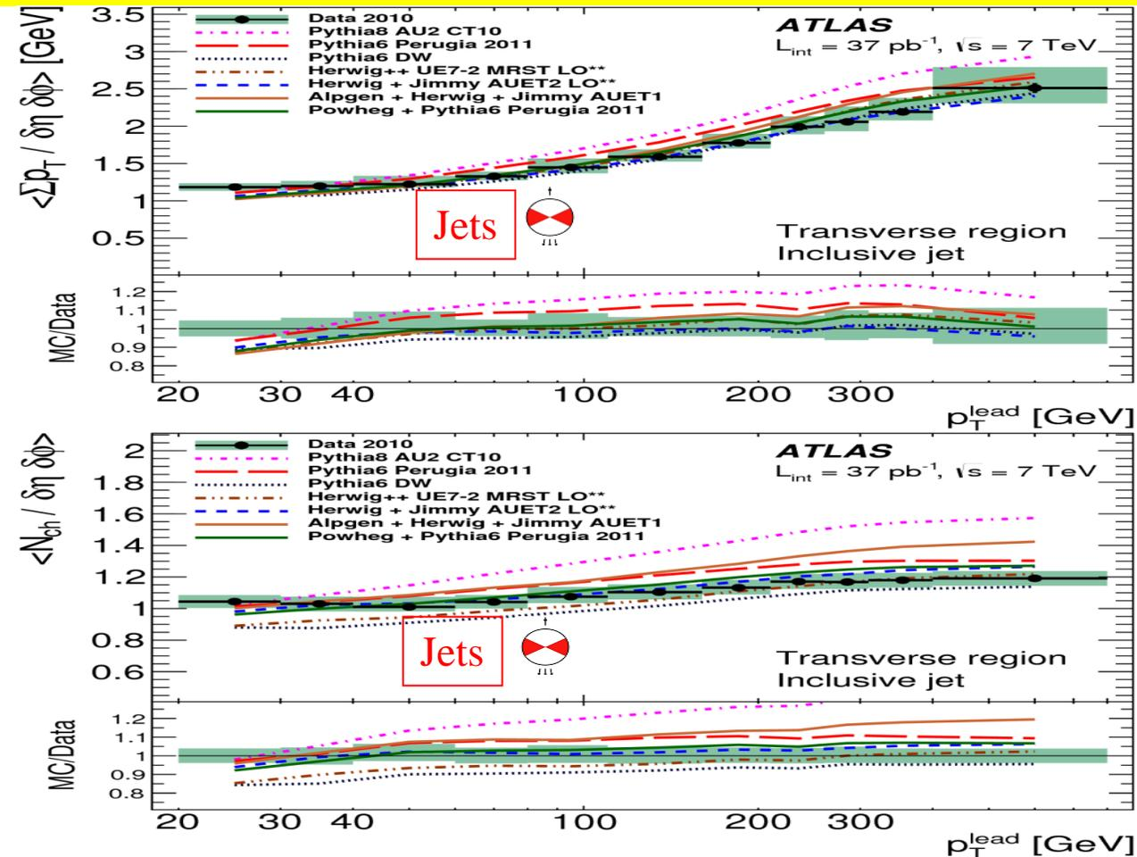
Comparison of particle level data and MC predictions for average scalar  $p_T$  sum density of tracks and average track multiplicity density values as a function of Z and leading jet transverse momentum.
