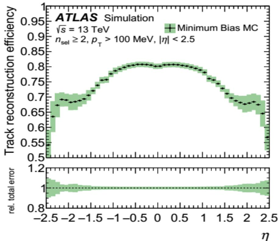
The primary track reconstruction efficiency integrated over  $p_T$  (left), integrated over  $\eta$  (middle) and as function of  $p_T$  and  $\eta$  (right). The green shaded error band includes the total systematic and statistical uncertainty
