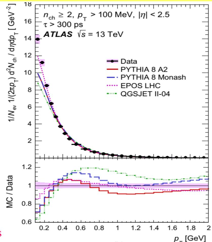
Primary charged-particle multiplicities as a function of  $p_T$  for events with  $n_{ch} \geq 1, p_T > 500 \text{ MeV}$  and  $n_{ch} \geq 2, p_T > 100 \text{ MeV}$  in  $|\eta| < 2.5$ .
