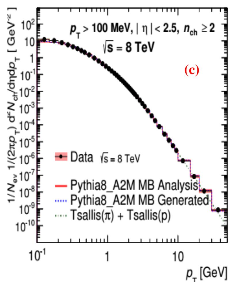
Charged-particle multiplicities as a function of the transverse momentum for events with  $n_{ch} \geq 2$ ,  $p_T > 100 \text{ MeV}$  and  $|\eta| < 2.5$  at  $\sqrt{s} = 0.9$  (a), 7 (b) and 8 TeV (c). The dots represent the data and the curves the predictions from different MC models.
