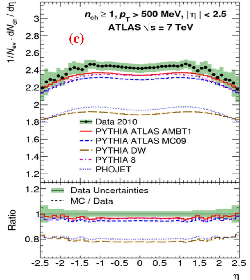
Charged-particle multiplicities as a function of the pseudorapidity for events with  $n_{\text{ch}} \geq 1, p_{\text{T}} > 500 \text{ MeV}$  and  $|\eta| < 2.5$  at  $\sqrt{s} = 0.9$  (a), 2.36 (b) and 7 TeV (c). The dots represent the data and the curves the predictions from different MC models.
