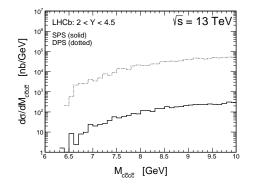
Rysunek: Distribution of invariant mass of four  $c - \bar{c}$  system. Here  $\sqrt{s} = 13$  TeV and each quark/antiquark rapidity is contained in the rapidity interval (2,4.5). The solid line is for SPS and the dashed line for DPS contributions.
