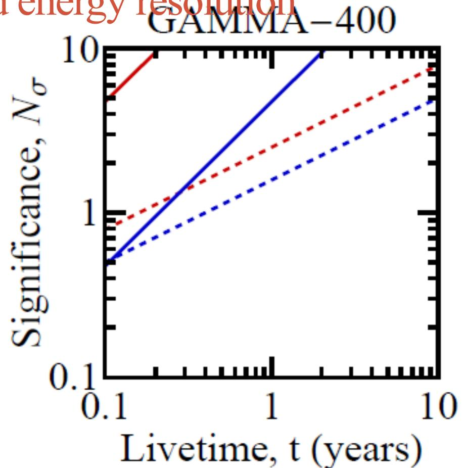
The expected significance of 135 GeV line in the flux spectrum (dashed lines) or the fluctuation angular power spectrum (solid lines) analysis of the diffuse  $\gamma$ -ray background with the Fermi-LAT or GAMMA-400 experiments.
