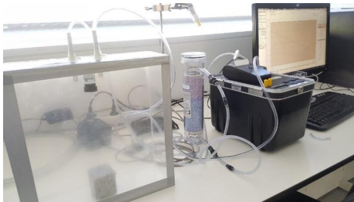
a) RAD7 detector with a closed loop arrangement.
