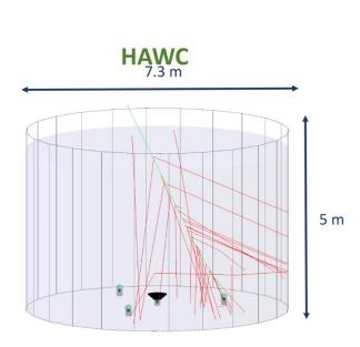
3x 8-inch PMTs 1x 10-inch PMT in the center of the tank Water height 4,5 m (5 m total height) Polypropylene walls
