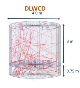
2x 8-inch PMTs Water height 3,75 m Tyvek walls
