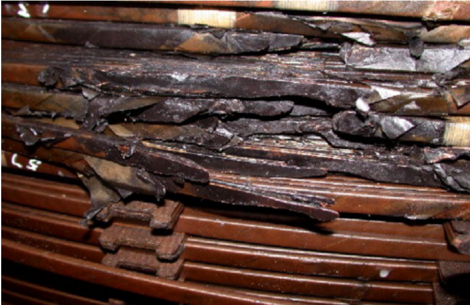
Failure in a 700 MVA generator transformer in South Africa after the Halloween storms of 2003. [Thomson et al., Adv. Space Res., 2010]
