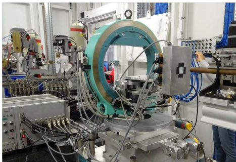
Fig. 4 - The Dual Plane Detector mounted on 5 axis automated stage. Is possible to see also the TAKES read out system.
