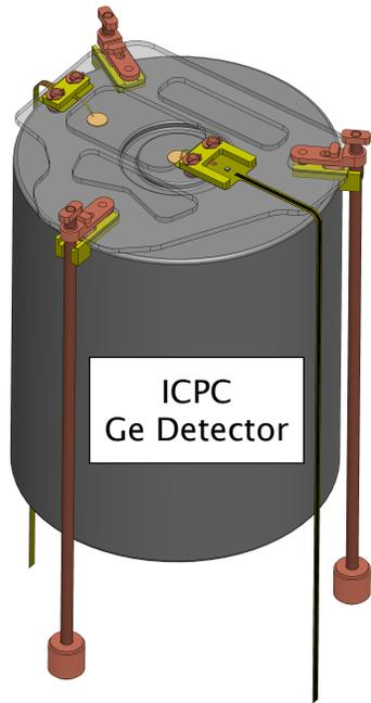
ICPC: Inverted-Coaxial Point Contact
