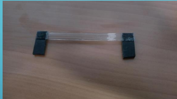
Figure18. Dummy optical fibre array. Produced to perform the tests.
