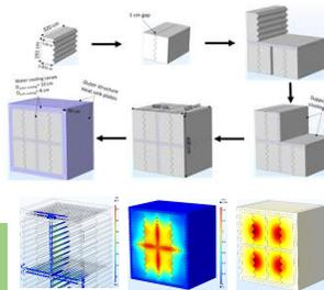
Fig. 7: Seg-blocks BD core assembly and thermo-structural performance.
