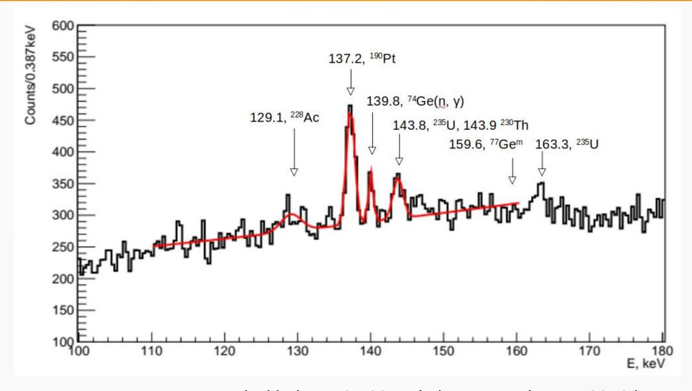
Energy spectra measured with the 148.122 g platinum sample over 8946 hours around the 137-keV region
