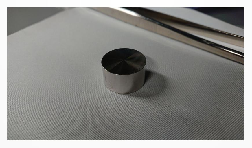
diameter 25.04(1) mm, thickness 14.07(2) mm, mass 148.122(1) g, purity grade is 99.95%
