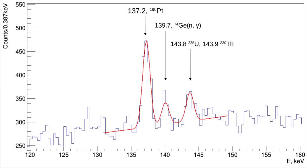
Energy spectra measured with the 148.122 g platinum sample over 8946 hours around the 137-keV region
