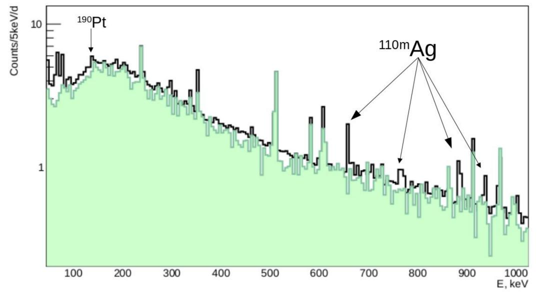
Energy spectra in the energy intervals 50 – 1000 keV measured with the platinum sample over 373 d (black line) and without sample over 28 d (filled green) both normalized to time (d)
