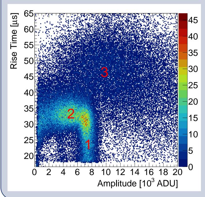
Pulse rise time versus amplitude in an 30 cm diameter SPC filled with 1.3 bar He:Ar: $CH_4$  (51.7%:46%:2.3%) and <sup>55</sup>Fe source inside the detector. The three distinct populations are (1) 5.9 keV photons interacting in the gas volume, (2) interactions near the cathode, and (3) cosmic muon interactions. Pulse-shape discrimination enables background suppression and fiducialisation.
