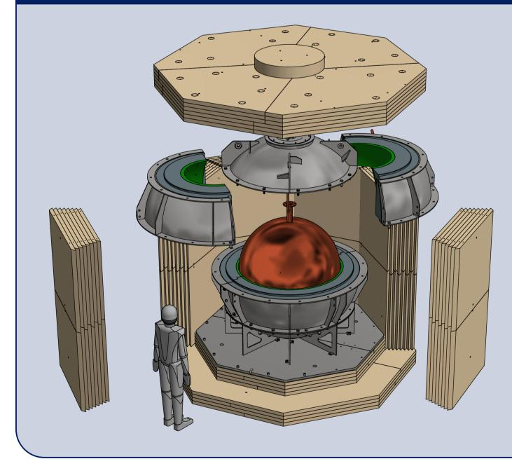
First results were obtained with SEDINE, a 60 cm diameter SPC operated in the Laboratoire Souterrain de Modane (LSM), and placed the first exclusion limits on a 0.5 GeV mass DM candidate with  $\sigma_{\rm SI} = 4.4 \times 10^{-37} {\rm cm^2}$  [2]. A 140 cm detector, SNOGLOBE, constructed using 4N copper with an electroplated internal layer to suppress background, was recently installed SNOLAB, Canada (left).
