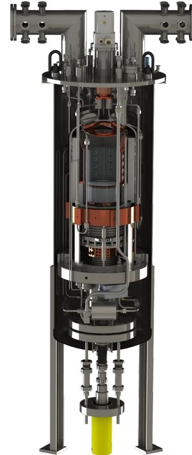
Inside the PV : cross sectional view of the fused silica jars and other controls
