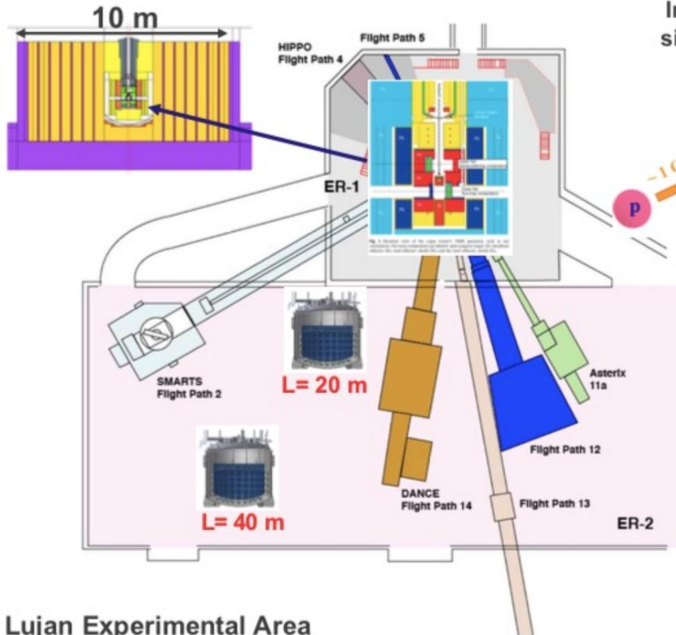
Intense source muon neutrinos: target MCNP simulation flux  $4.74 \times 10^5 \nu/\text{cm}^2/\text{s}$  at 20 m
