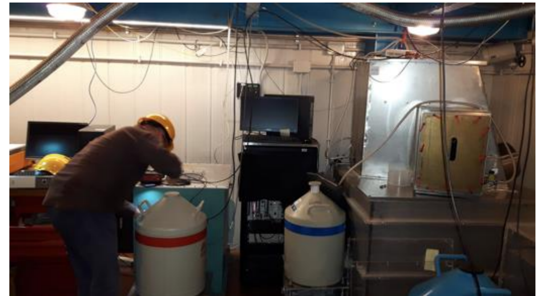
Connection of the Front-End electronic to the BEGe's Canberra preamplifier (Mod. 2002C), behind the liquid N2 dewar
