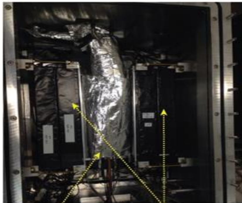
heat insulator wrapped around the SDDs
