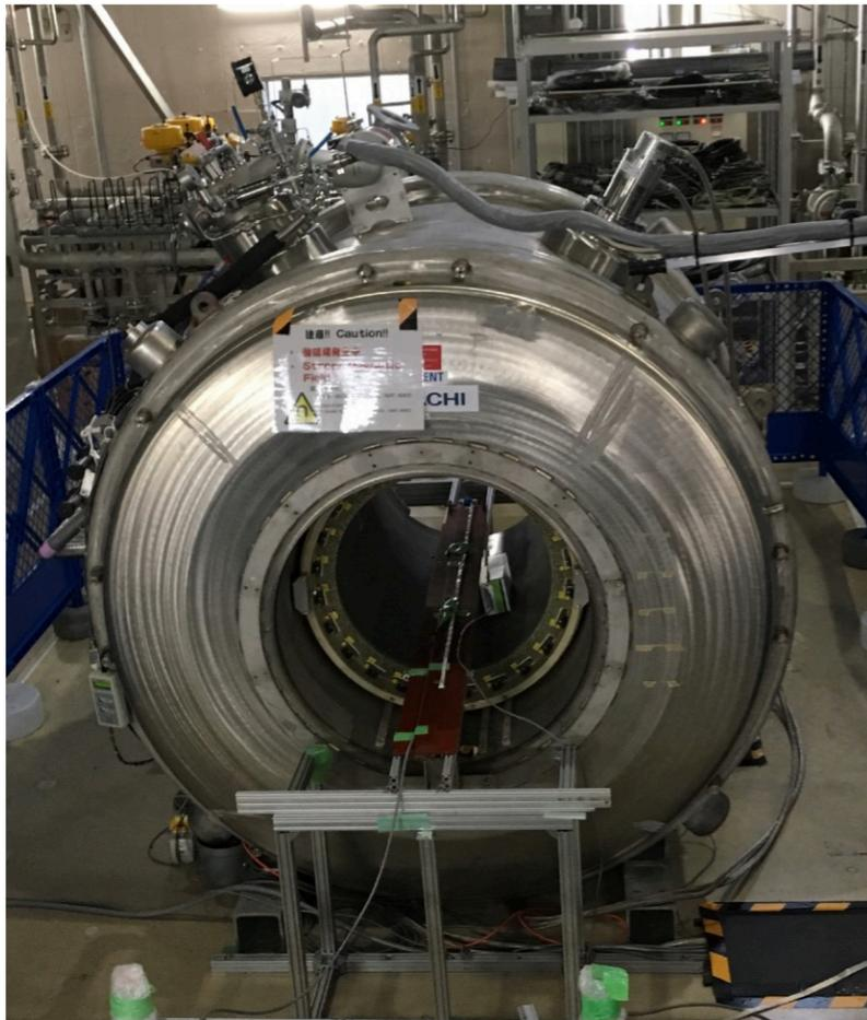
Superconducting Magnetic field : 1.7T
