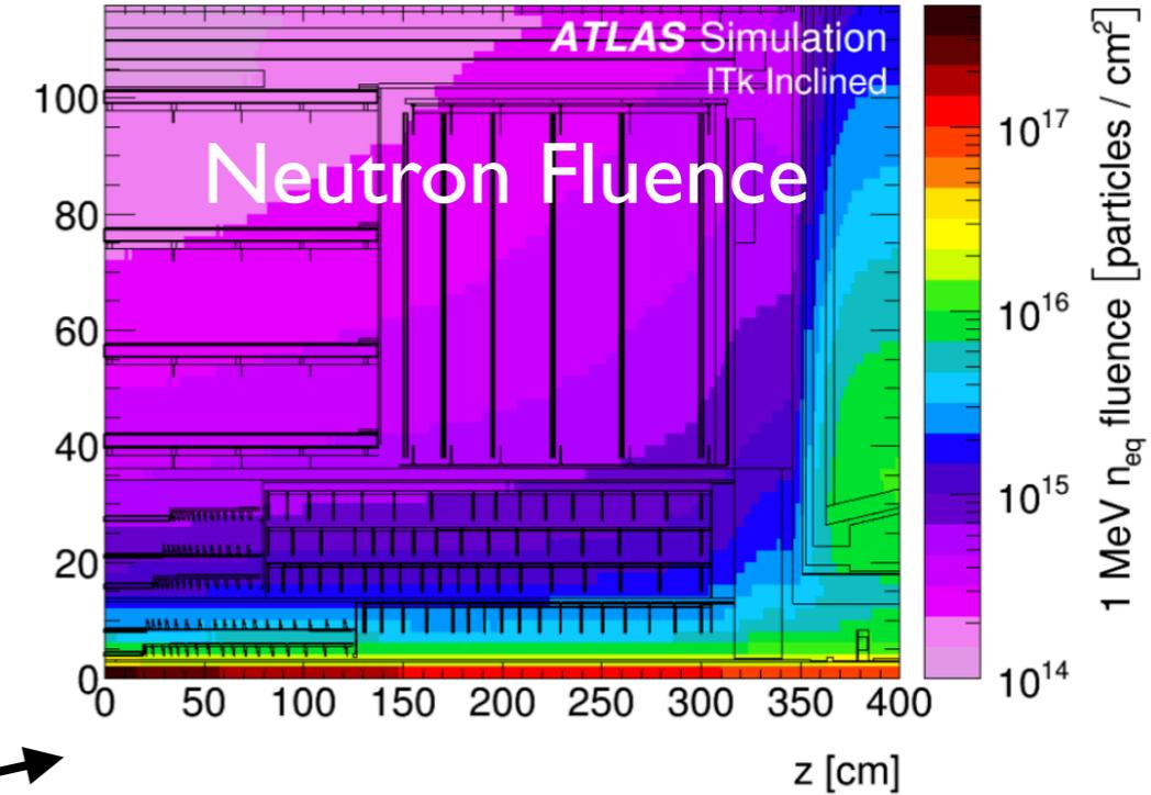
Sensor, electronics and mechanical must survive to 4000  $ab^{-1}$   $\sim$  10x nominal LHC
