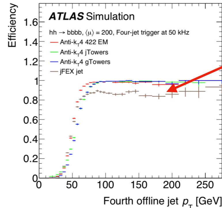
Full detector allows for more anti- $k_T$  like algorithm that improves near by jet efficiency
