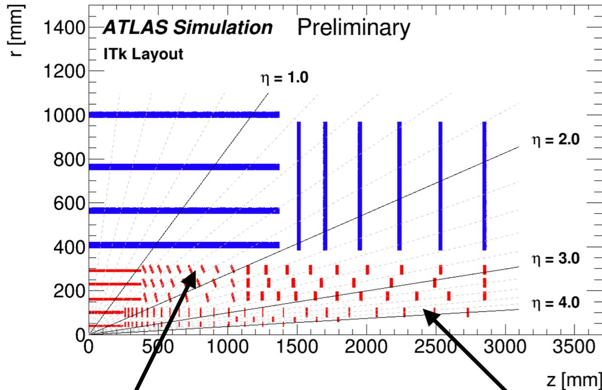
Inclined sensors provide shorter path length of particles through overlap region sensors
