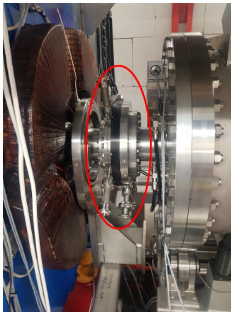
Figure 11: A photo for one Rogowski BPM installed in COSY.
