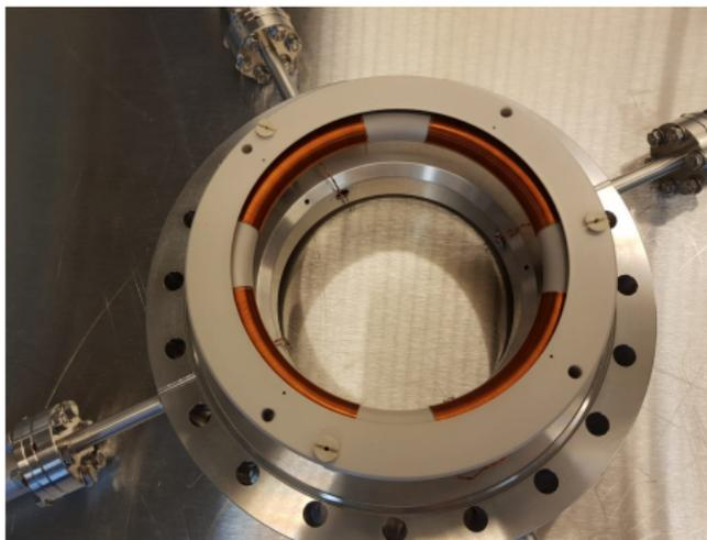
Figure 7: Rogowski BPM winding with incomplete angular range.
