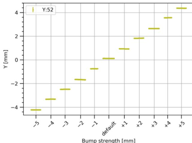
Figure 12: Vertical orbit measured by Rogowski BPM after applying a local orbit bump.
