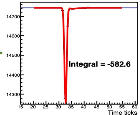
Pulse width:  $\sim 500\text{ps}$ , Pulse amplitude:  $\sim -100\text{mV}$
