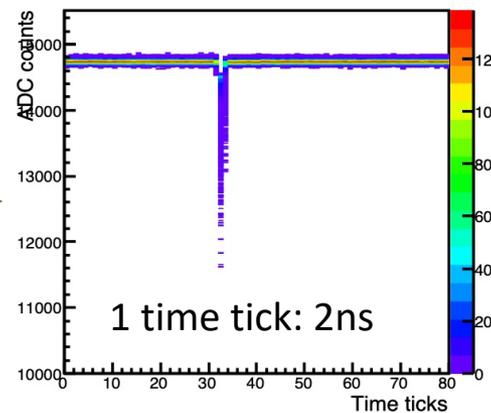
Extracted average pulse shape and charge
