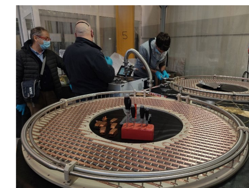
BP leak tests
