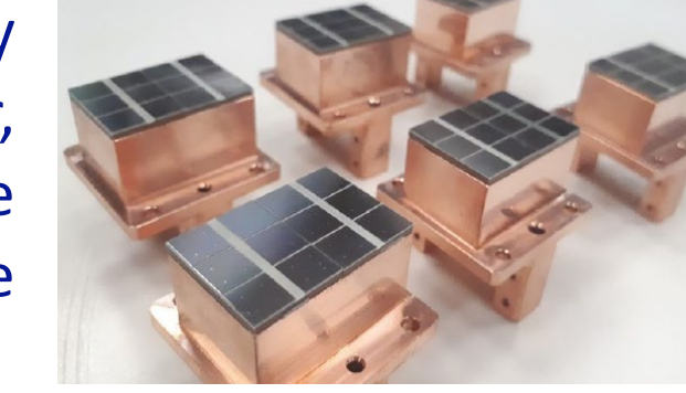
FEE holders with glued SiPMs
