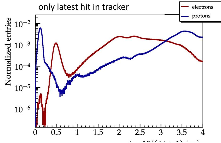
the two populations (electrons and protons) are clearly distinct  $\rightarrow$  the e/p identification capability seems confirmed and seems also improving with energy
