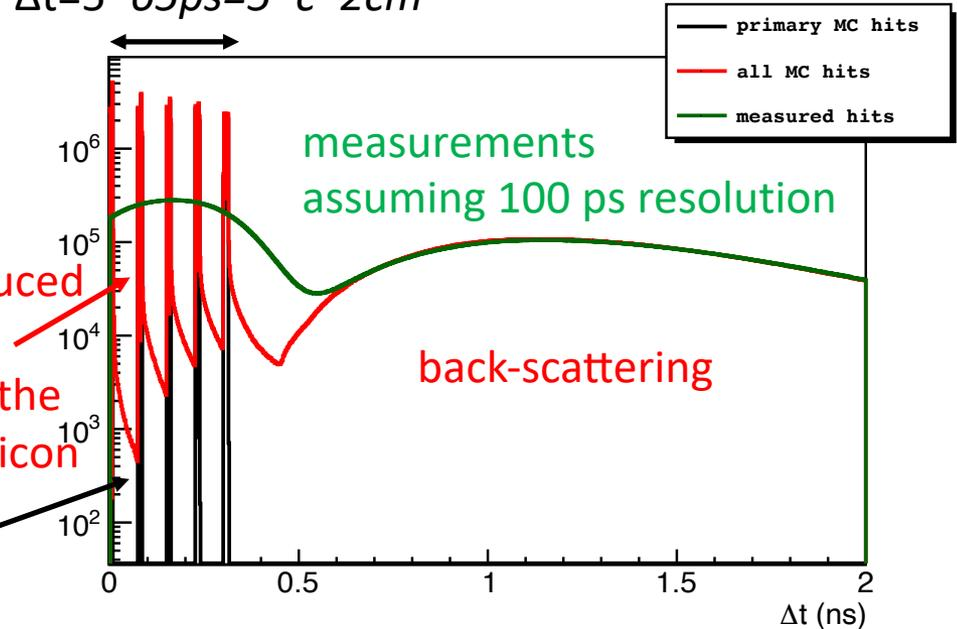
$O(100\text{ps})$  timing resolution enables to separate back-scattering from primary hits in the tracker  $\rightarrow$  improved efficiency in track reconstruction
