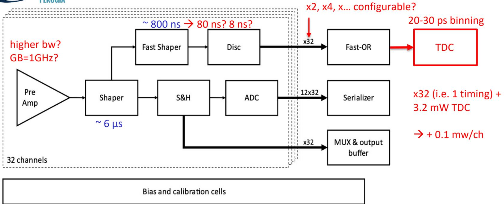
Figure 3 ASTRA 32-channel architecture
