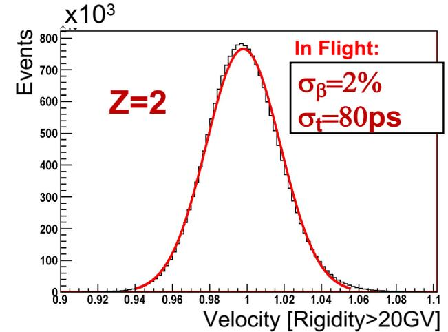
**Measures Velocity and Charge of particles**
