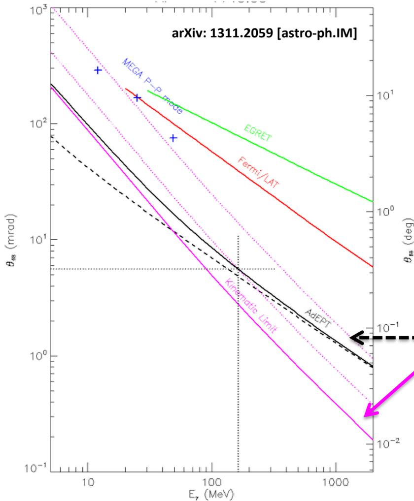
The angular resolution of a pair-conversion telescope:
