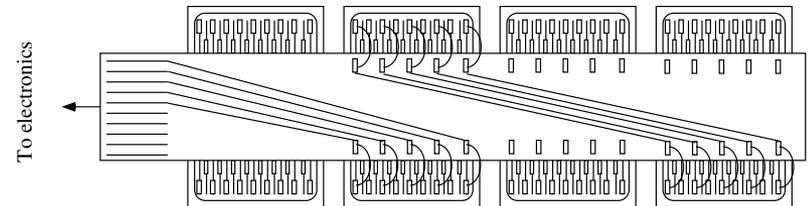
"multiplicity" (or "ambiguity"): the 1500-3000 K-side channels needed for each ladder are "merged" into 384.
