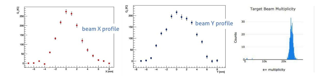
The target was designed for 5000  $e^+$ /bunch, but behaves **linearly** even at 35000  $e^+$ /bunch (working region 20k-30k  $e^+$ /bunch)
