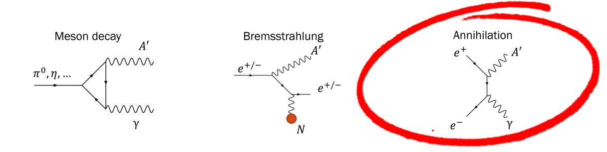
An  $e^+$  beam at E<550 MeV is fired on a 100  $\mu$ m thick diamond target to produce a visible photon  $\gamma$  and a dark photon A'
