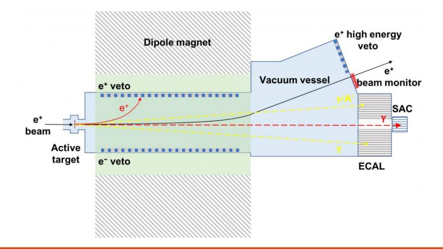
**Electron-positron annihilations** occur in a 100  $\mu$ m thick, 2x2 cm<sup>2</sup> large, CVD grown **diamond active target**.
