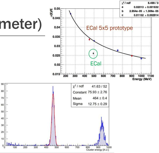
First calibration performed on prototype (5x5 crystals, solid line in plot)
