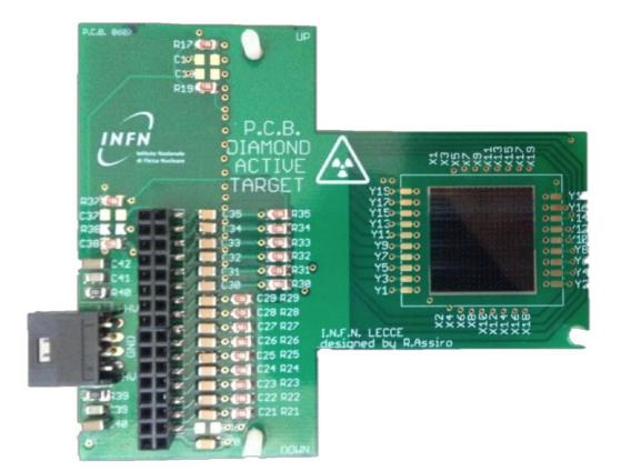
Electron-positron annihilations occur in a 100  $\mu m$  thick, 2x2 cm² large, CVD grown diamond active target.
