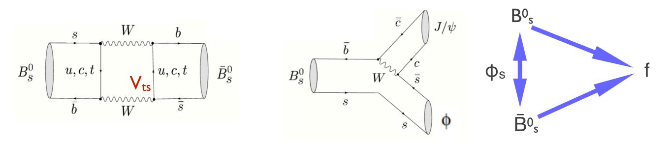
Golden channel:  $B^0s \rightarrow J/\psi \phi \rightarrow \mu^+\mu^-K^+K^-$ : proceeds (mostly) via a b $\rightarrow c\bar{c}s$  tree diagram
