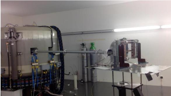
Acrorad and EURORAD CdTe detectors tested at ICNAS, Coimbra, cyclotron proton beamline.
