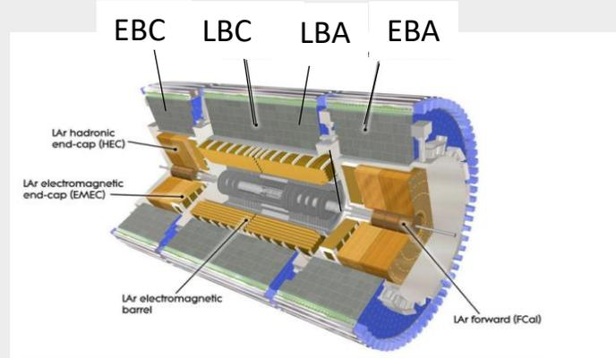
Fig. 1. A cut-away view of the ATLAS calorimeters. The Tile Calorimeter consists of one central barrel and two extended barrels. [2]
