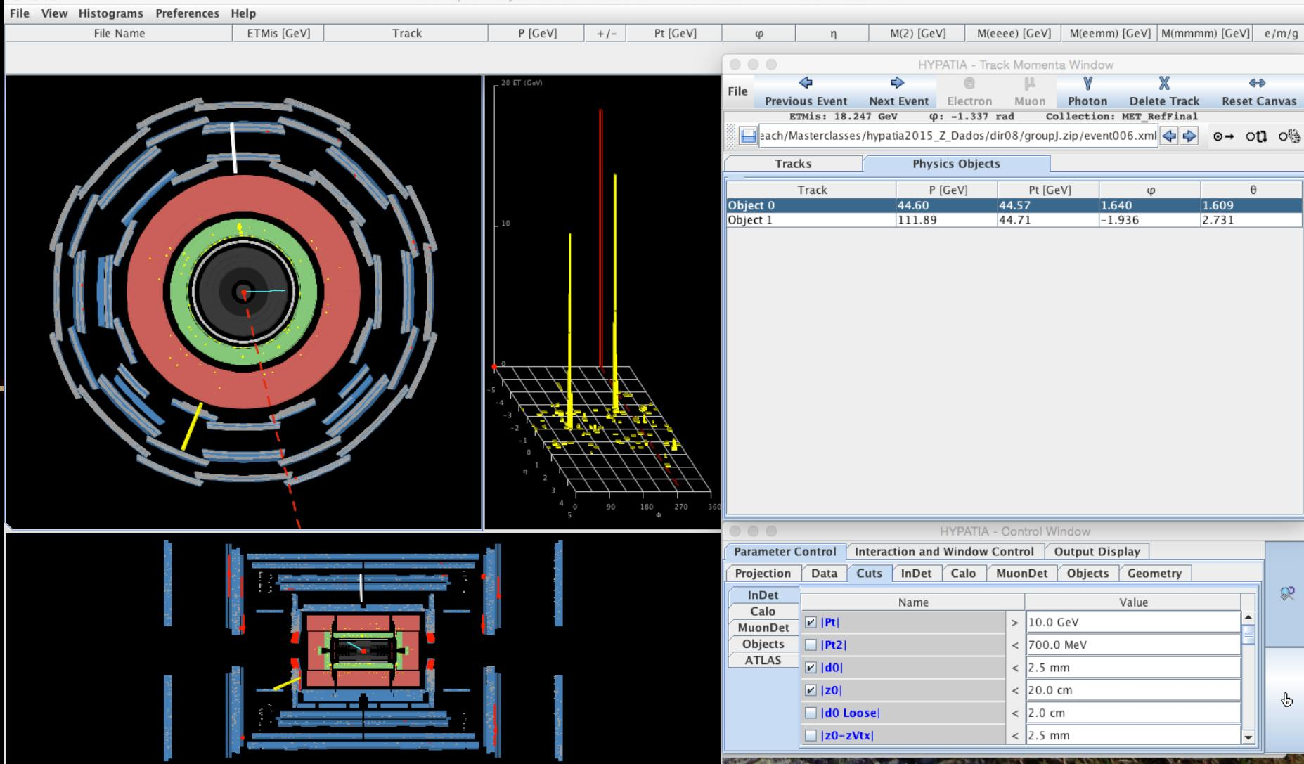
Photons are neutral particles; they do not leave tracks in the inner detector; only energy deposits in the electromagnetic calorimeter.
