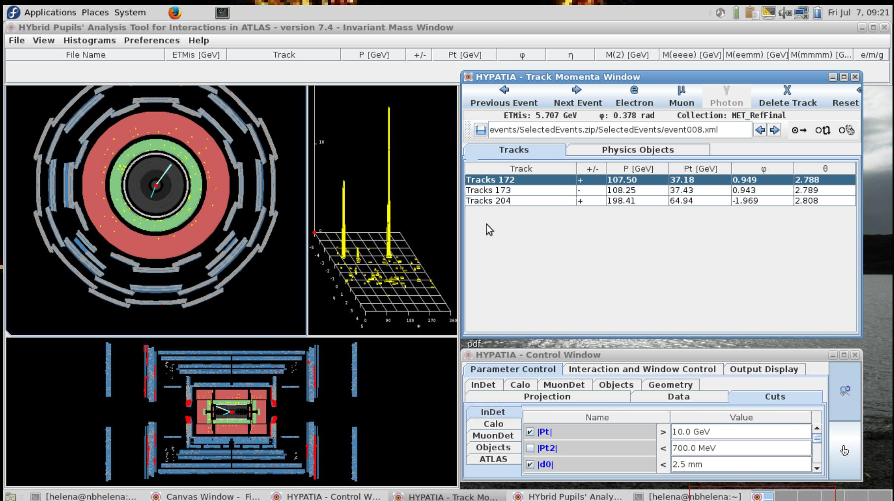
The cut in the  $p_T$  (transverse momentum - the linear momentum projected in the transverse plan of the detector) allows the low- $p_T$  track removal, which helps to improve greatly the signal to background ratio.
