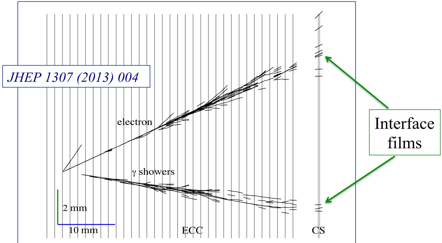
a  $\pi^0$  is produced at the primary interaction vertex and a  $\gamma$  is detected
