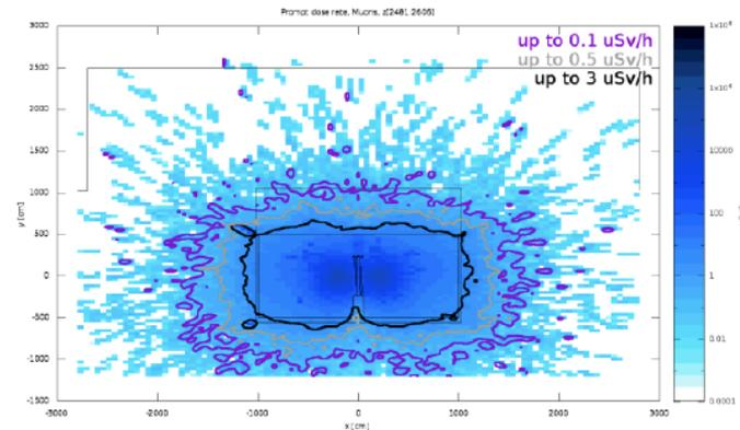
Updating simulations with 1m of concrete roof
