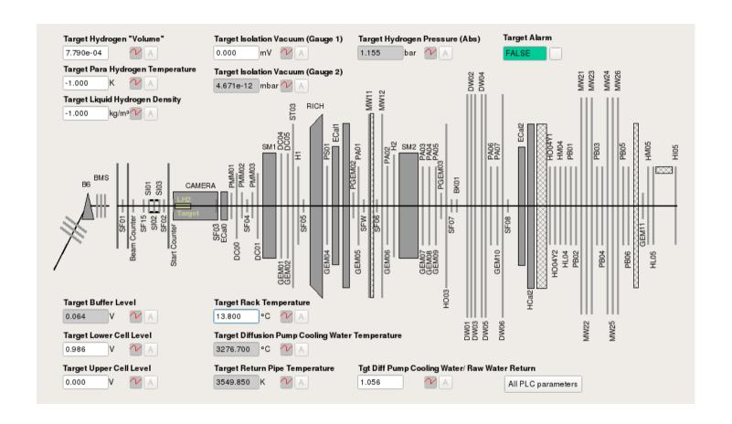
Connection to Siemens S7-1200 PLC via S7 driver
