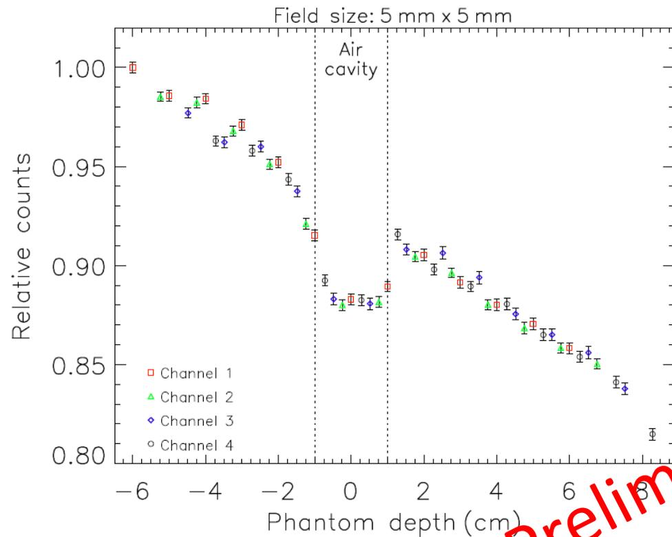
Background subtraction allows to increase the detectability of the air cavity
