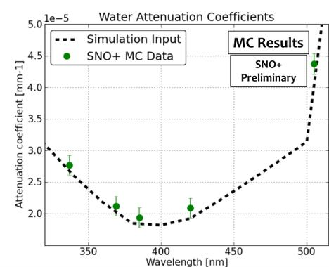
PMT Angular Responses and Water Attenuation coefficients from MC Laserball data.
