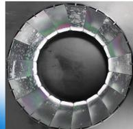
PMT Angular Response changes with time due to degradation of the PMT reflectors.
