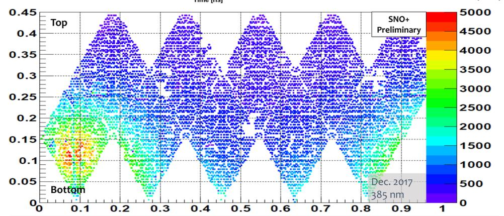
Cosahedron projection of the SNO+ detector. Shows the number of hits in each PMT, with the Laserball at the bottom of the detector.
