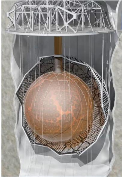
SNO+ consists of a large volume liquid scintillator detector located 2 km underground at SNOLAB, Sudbury, Canada. It reuses most of the components of the SNO detector.
