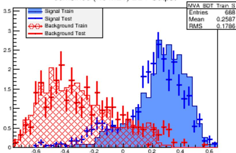
*BDT test (points) and train (filled histogram) sample outputs for signal (blue) and background (red).*
