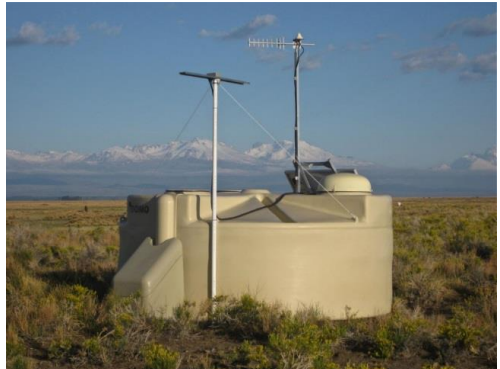
Figure 1: Cherenkov water tanks for cosmic rays detection
