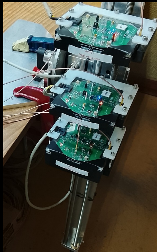
Muon telescope for classes and outreach
