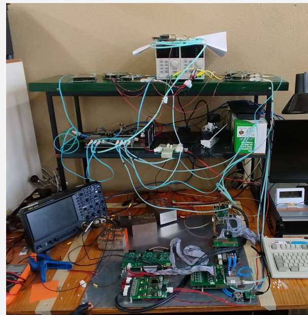
Distributed DAQ for TOMAR. Tested with a dummy detector
