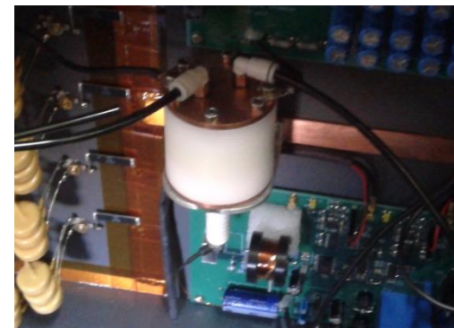
Spark gap modified by user => chamber destroyed
