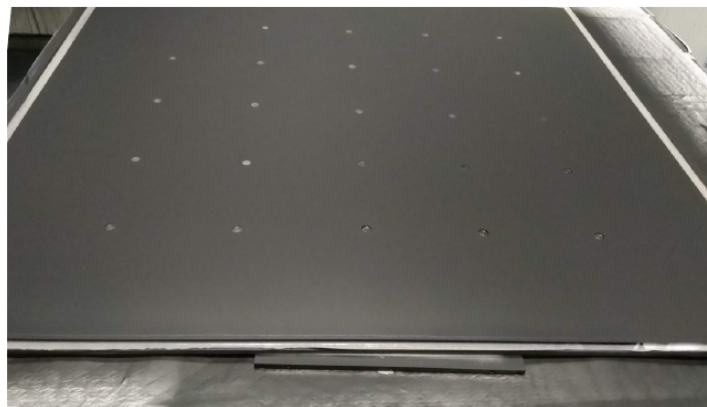
Multi-gap assembly: 5x5 spacer matrix + peripheral strip all around the gaps for sealing.
