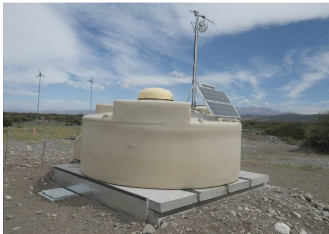
RPC deployed on the AUGER site under water Cherencov tank
