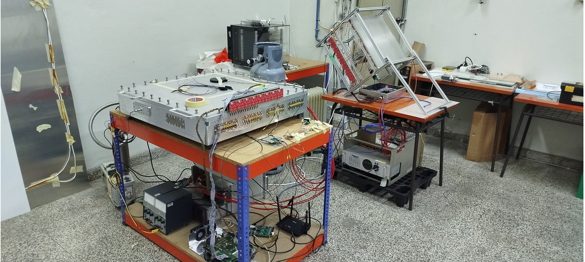
Hipo-barc chamber with capacity to hold 4 RPC planes
