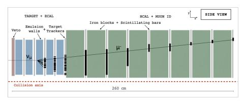
• Electronic Calorimeter and Target: Composed of emulsion Tungsten walls and scintillator fibers, it follows the electromagnetic showers with a temporal and spatial profile.
