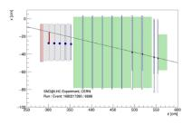
Each Upstream (US) (5 first planes) hit has a QDC value that allows for the distinction between single muon background and dimuon signal.
