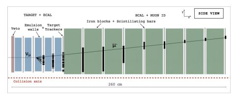
• Hadronic Calorimeter and Muon System: Composed of Iron walls and scintillator bars, it develops the hadronic showers, detects their energy and identifies muons leaving the detector.
