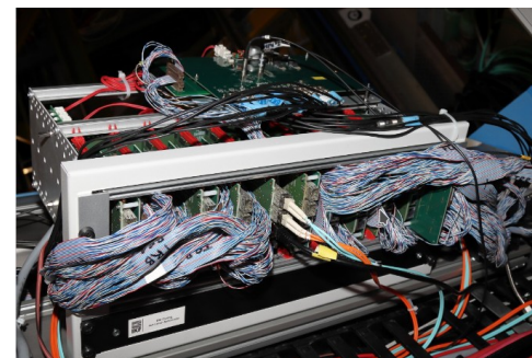
DAQ parts of HADES detector
