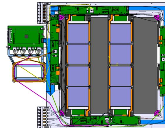
**Silicon station geometry layout**
