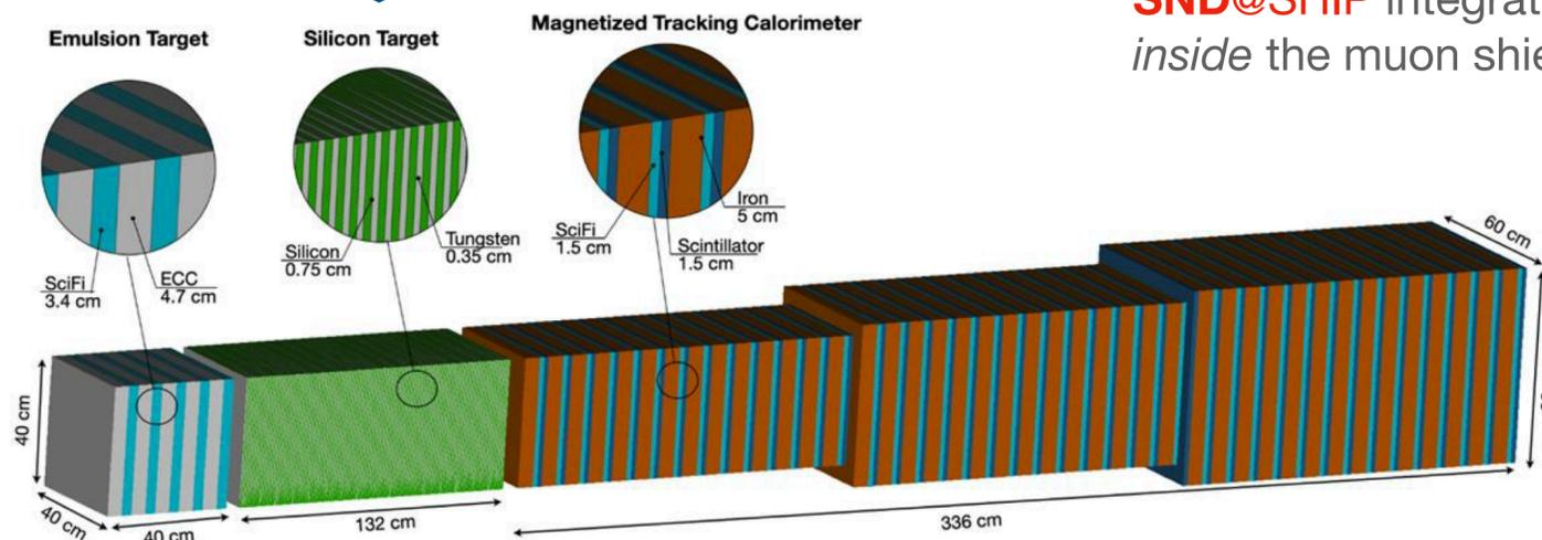
SND@SHiP integrated inside the muon shield
