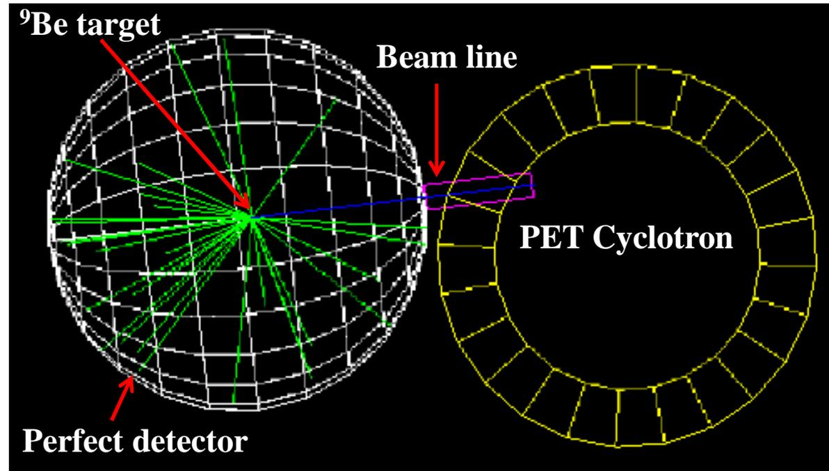
A proton beam with 18.5-MeV energy was shot in vacuum through a 25.2- $\mu\text{m}$ -thick  $^9\text{Be}$  target
