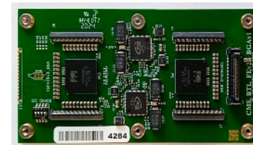
Figure 3. BTL front-end board (left); BTL time resolution vs integrated luminosity (right).
