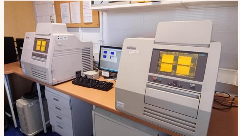
Figure 2: Harshaw 6600E TLD readers used to analyze LiF:Mg,Cu,P detectors and measuring H_p(3) .
